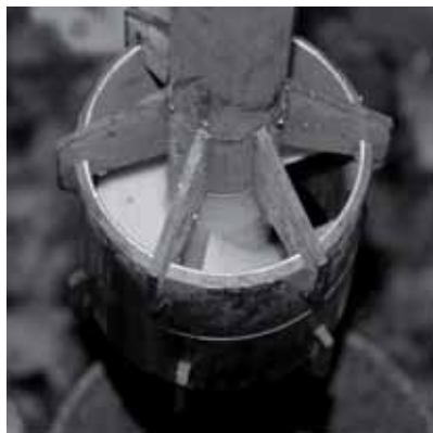
Figure 6.1: Nose of the Haferland flow meter where the propeller is installed. Foto: René Kaufmann
